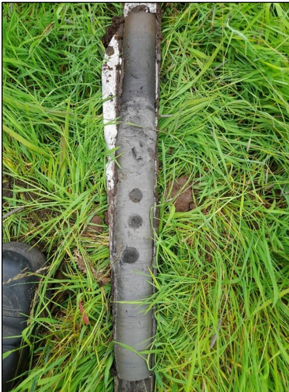
Photograph 2 - Russian Core taken at RG1P2 (Peat Area 2). Depth 0.75m-1.15m. Showing more decomposed peaty loam topsoil (0.75m-0.9m and clay (0.9m-1.15m). Water table detected beneath this at 1.15m
